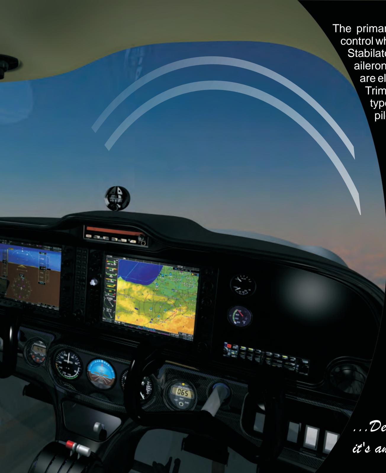
The primary flight controls are of conventional type operated by control wheels and rudder pedals.
